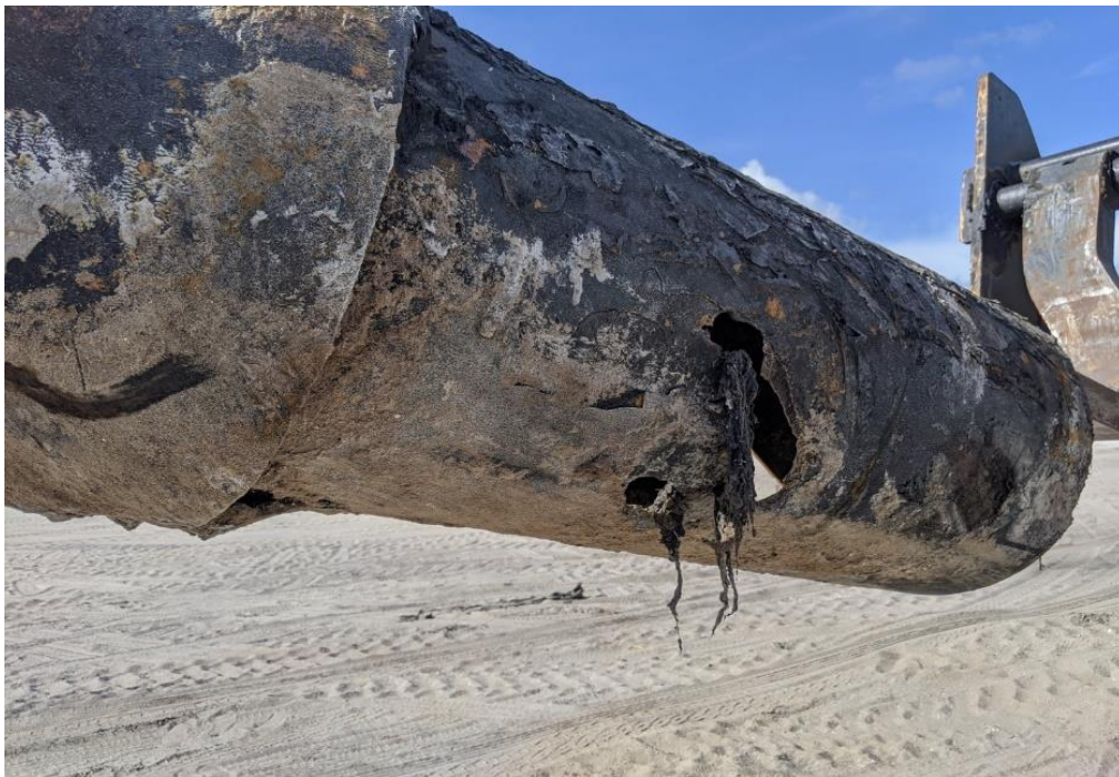
Figure 1-1 Photograph of Existing Force Main Leak
