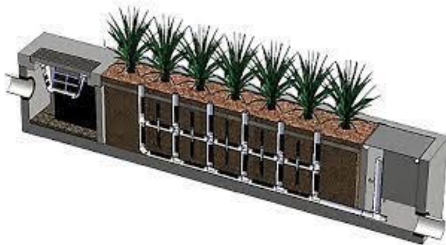
Figure 4: Modular / Linear Wetland System Schematic
