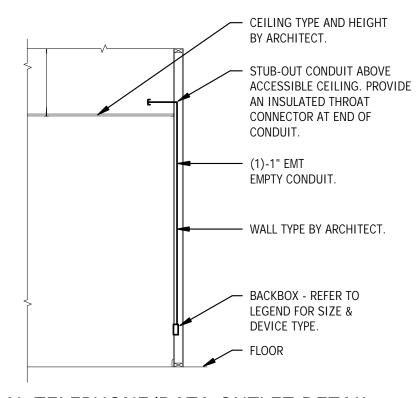
TYPICAL TELEPHONE/DATA OUTLET DETAIL SCALE: NONE
