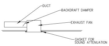
EXHAUST FAN DETAIL SCALE: NONE
