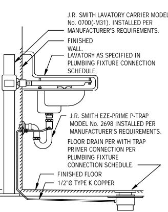
PIPING ARRANGEMENT SHOWN IS SCHEMATIC. ADJUST TO SUIT FIELD CONDITIONS. MAKE TRAP PRIMING PIPE SAME SIZE AS EZE-PRIME FITTINGS. FOLLOW MANUFACTURER'S INSTRUCTIONS FOR INSTALLATION PROCEDURE. TRAP PRIMER CONNECTION FROM COUNTERTOP MOUNTED SINK OR LAVATORY IS SIMILAR. VERIFY PROPER OPERATION WHEN INSTALLED.
