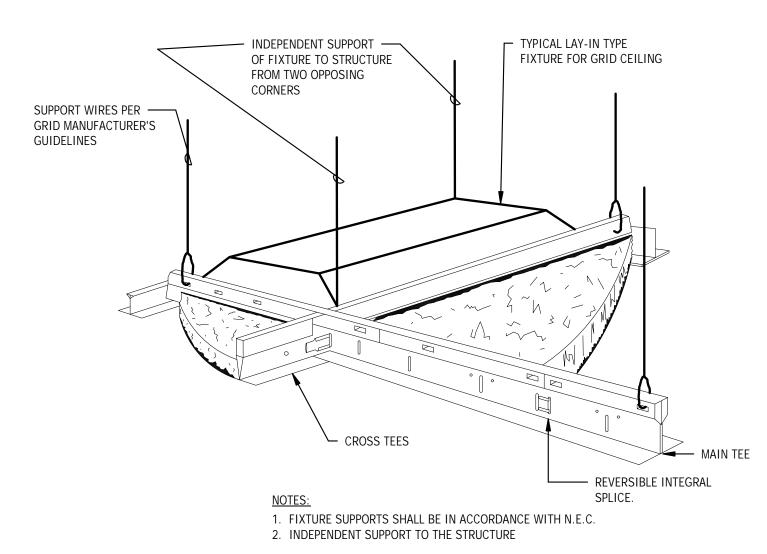
LUMINAIRE MOUNTING - ACOUSTICAL TILE CEILING SCALE: NONE
