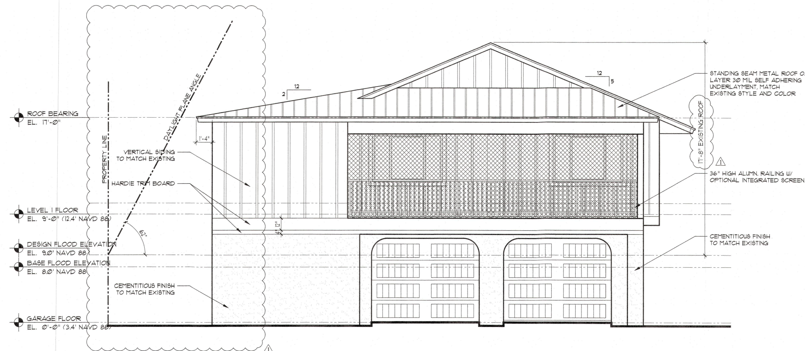
1 PROPOSED FRONT ELEVATION SCALE : 1/4" = 1'-0"
