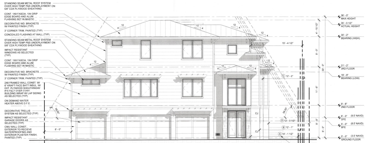
EAST (FRONT) ELEVATION 3/16" = 1'-0"
