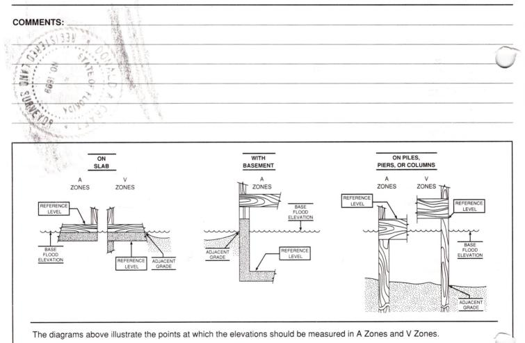
Elevations for all A Zones should be measured at the top of the reference level floor.
