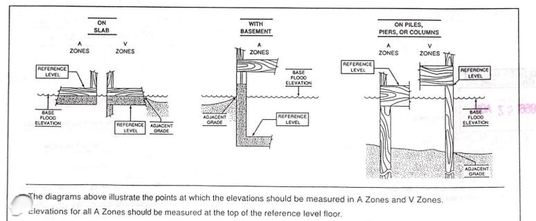
Elevations for all V Zones should be measured at the bottom of the lowest horizontal structural member.
