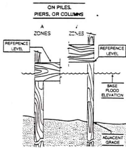
The diagrams above illustrate the points at which the elevations should be measured in A Zones and V Zones. Elevations for all A Zones should be measured at the top of the reference level floor. Elevations for all V Zones should be measured at the bottom of the lowest horizontal structural member.
