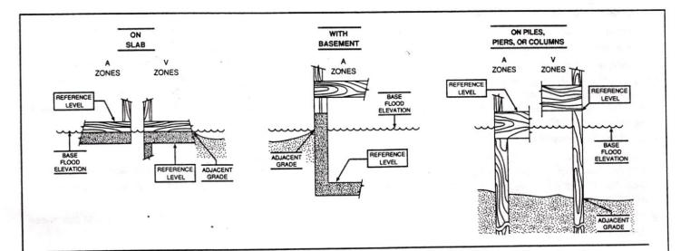
The diagrams above illustrate the points at which the elevations should be measured in A Zones and V Zones.
